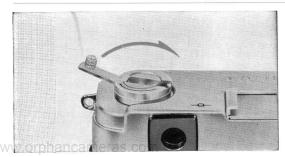
Flip up the film rewind crank handle to the horizontal position and gently wind in the direction of arrow until you feel a slight resistance.
