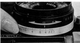
After determining the ASA speed of the film loaded in camera and the distance (feet or meters) from subject to camera, read the correct flash number on top of this feet (or meter) number.
