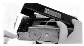
Open the Back Cover by pulling down on the Back Cover Locking/Unlocking Bar and it will swing open. Open fully by hand.
