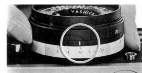
When you use the External BC or Electronic Flash, camera must be set for manual control. Exposure settings for these external flash units are determined according to instruction accompanying them.
