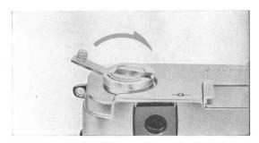
Flip up the Film Rewind Crank to the horizontal position and wind in the direction of the
