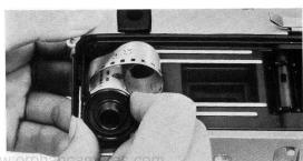
Insert a new 35mm film cassette in Film Loading Chamber.
