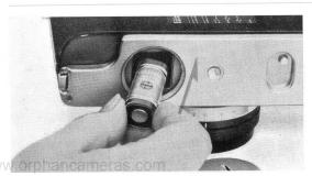
Insert a new battery with plus (+) terminal facing top of the compartment.
