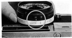
Be sure to set the ASA Index Number of the film loaded in camera and "AUTO" opposite the white diamond (as shown left) by turning the ASA Film Speed Contol Ring and AUTO and Manual Control Ring.
