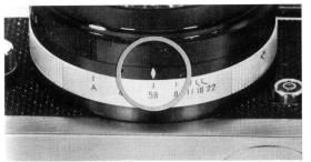
Manual Control of the aperture is achieved by turning the AUTO and Manual Control Ring clockwise to the desired flash number or corresponding F. stop engraved on the bottom of the Control Ring.
