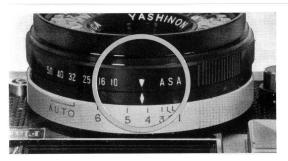
Then set the ASA Index Number of the film loaded in the camera opposite the "white diamond" (as shown left) by turning the ASA Film Speed Control Ring.
